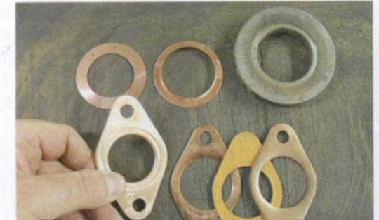
13 Pipe-join gasket (bottom left); die for forming it (top right); components
