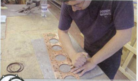
9 Dobson craftsman Dave Capstick forms the cylinder seal rings in the gasket
