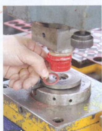
15 Punching out centre of fibre washers
