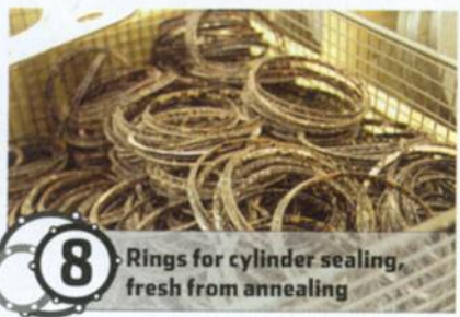
8 Rings for cylinder sealing, fresh from annealing
