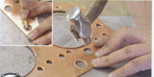
10 Forming the rings with a brass tool (inset); Dave forms cylinder seal rings in gasket
