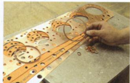
7 Head gasket bits: metal outer sheets, two inners, rings
