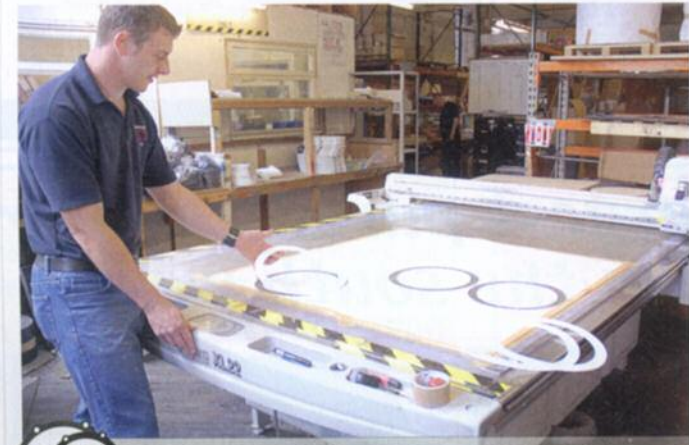
16 Computer-controlled cutter handles rigid sheet plastics
