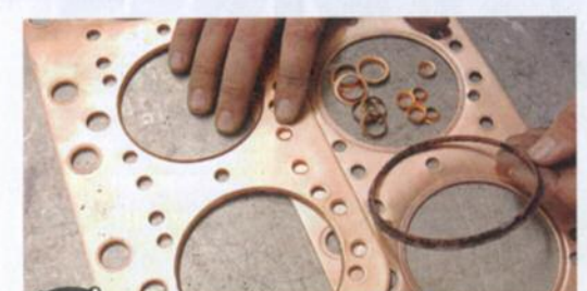
12 Part-assembled gasket (left); and that's the finished item on the right
